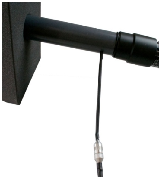
Fig. 18: Probe connected to the extension pipe.
