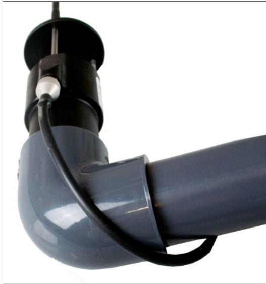
Fig. 18: Probe connected to the extension pipe.
