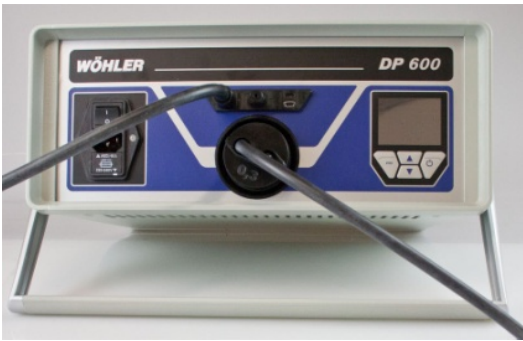
Fig. 12: Connection of the pressure tube and the air tube to the Wöhler DP 600
